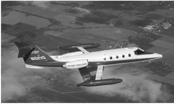
Fig. 1 Variable stability Learjet 25 (Calspan photo).
